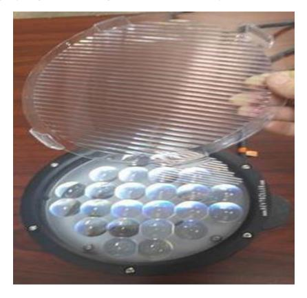
Picture of the spot light with the snap on lens to convert the spot into a straight line at no extra charge. The line only works to about 30 feet down or out. If you have a crane higher than 30 feet, we suggest you use the spot light, which will show up effectively on cranes up to 100 feet high.
